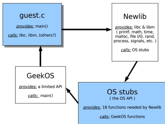
Figure 1: System software components and their dependence relationships
