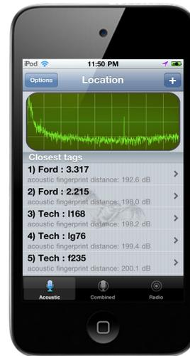
Figure 1: Apple iPod Touch running our Batphone localization software.
