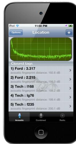
Figure 1: Apple iPod Touch running our Batphone localization software.
